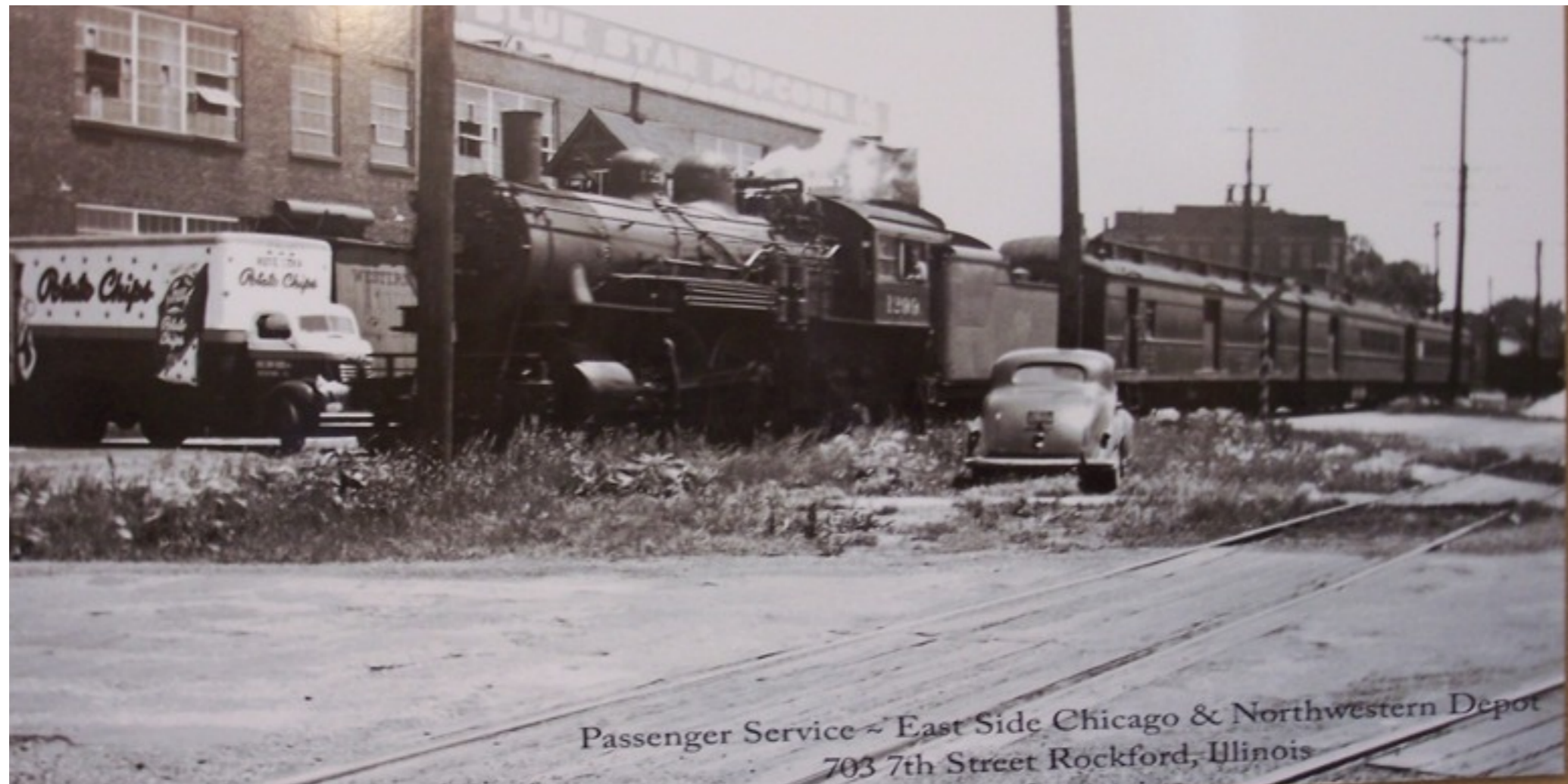
A photo from the 1940's of #1299 a 4-4-2 built by Schenectady. The passenger train has stopped at the Rockford 7th street station.
